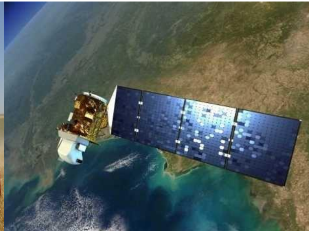
Landsat 8 providing multispectral image data at 30 m spatial resolution and 16 day repeat coverage.
